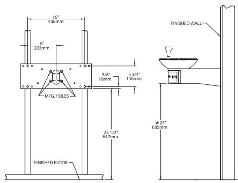
\*ADA REQUIREMENT NOTE - AFTER INSTALLATION, THREADED RODS MAY NEED TO BE TRIMMED
